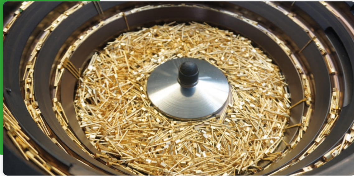
Bowl feeders specially designed for the material – in this case gold-plated contacts – separate and convey the parts using vibration and air pressure
